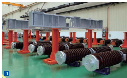
252kV Disconnector under assembly
