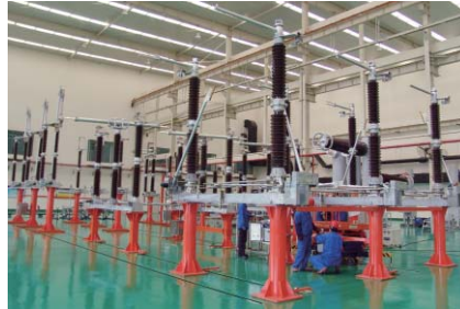
252kV Disconnector under assembly
