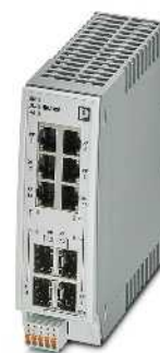
4/12 puertos RJ45, 2 puertos SFP y 2 puertos Combo Gigabit 10/100/1000 MBit/s
