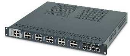
24 puertos RJ45 y 4 puertos Combo Gigabit (SFP o RJ45)
