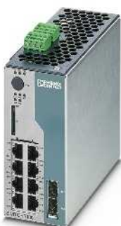
6 / 4 puertos RJ45 y 2 / 4 puertos Combo Gigabit (SFP o RJ45)
