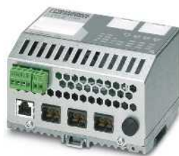
1 puerto RJ45 y 3 puertos POF SC-RJ
