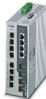
8 puertos Power over Ethernet RJ45, 4 puertos RJ45 y 4 puertos SFP
